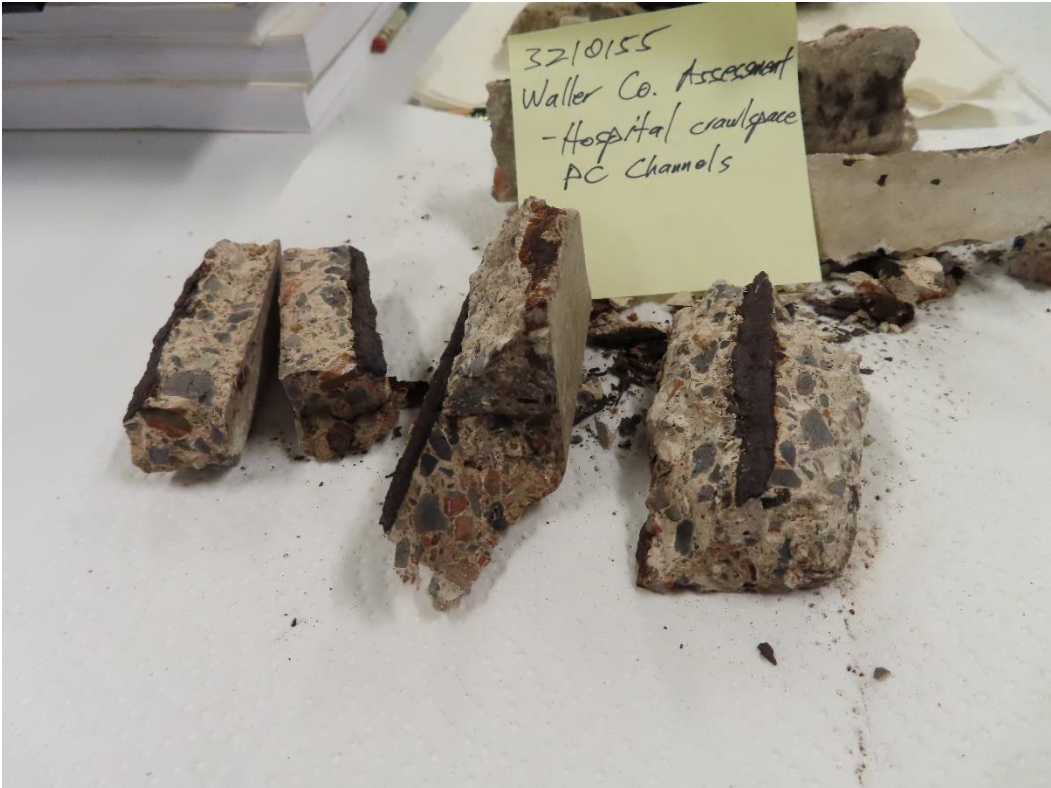
Photograph 21 – pH test results showing a pH less than 8.5.
