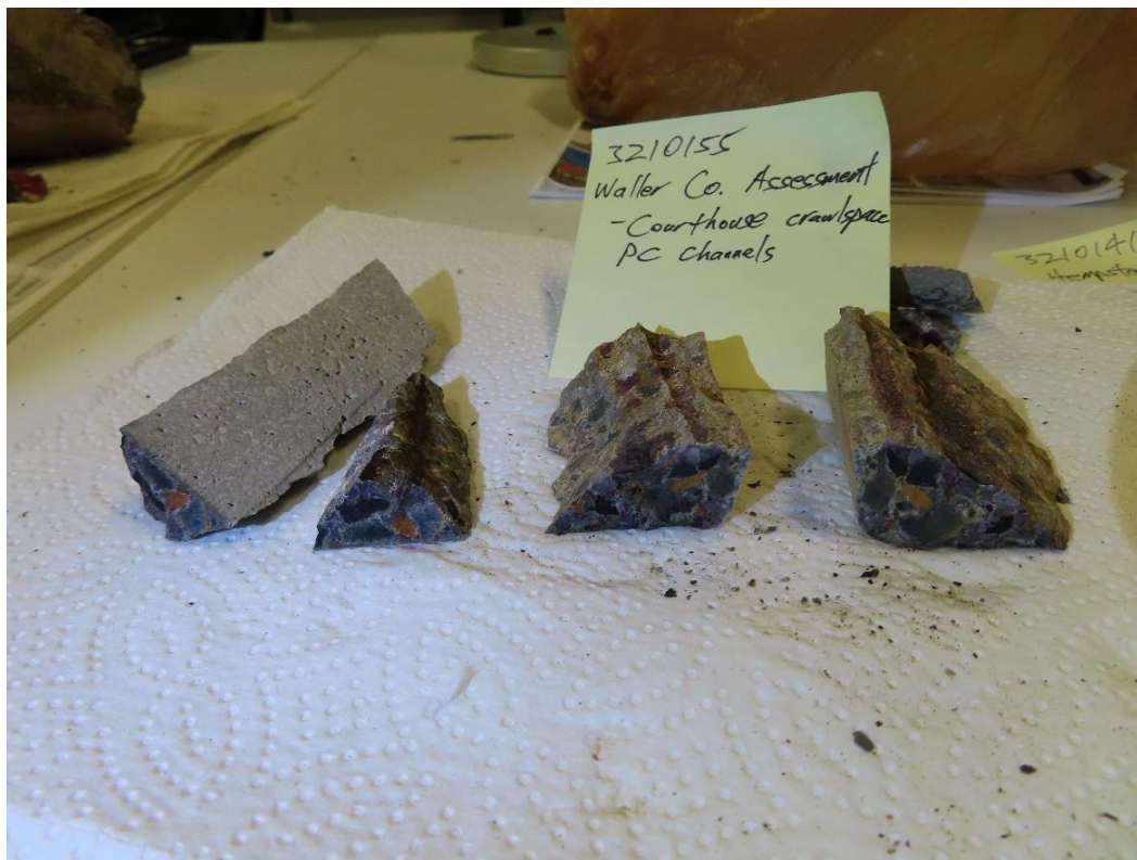
Photograph 6 – pH test results showing a pH less than 8.5.
